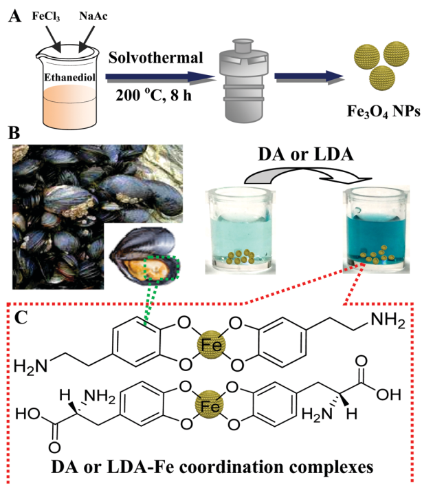
Scheme 1 (A) The synthesis procedure for mesoporous \text{Fe}_3\text{O}_4 NPs by a solvothermal route; (B) the mussel-inspired enhancement of \text{Fe}_3\text{O}_4 NP catalysis upon adding DA or LDA; (C) the molecular structures of DA and LDA and their bis-catechol-Fe coordination complexes formed on \text{Fe}_3\text{O}_4 NPs.
